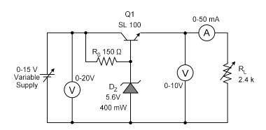
Fig. 1 Circuit diagram of series regulator
