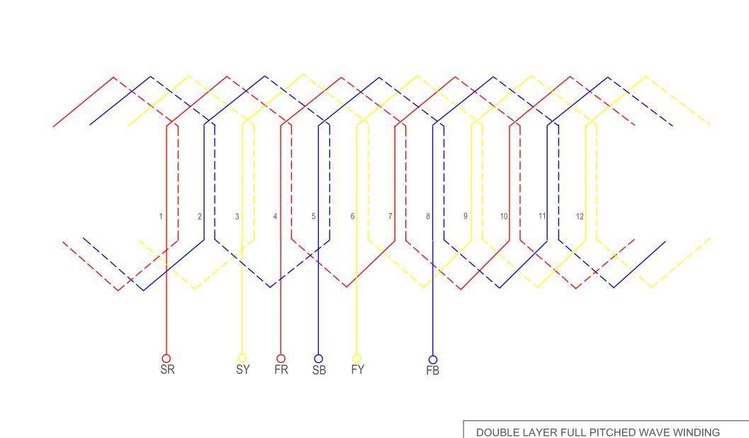
DOUBLE LAYER FULL PITCHED WAVE WINDING 3 PHASE, 12 SLOT, 4 POLE
